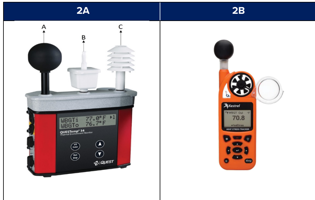
Figure 2A: An example of a standard WBGT device with black globe, wet bulb, and dry bulb thermometer attachments.
