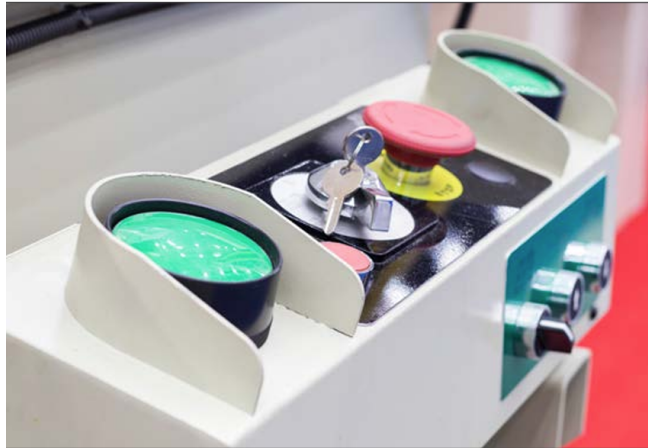
Green switches need two hands to operate
