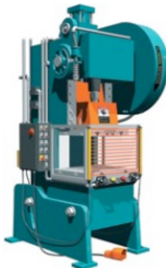
Figure 14: Machine safety curtain installed
