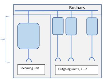
Figure 6-1 Internal Separation
