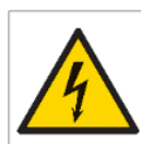
Figure 3-1: A typical warning label for live electrical equipment
