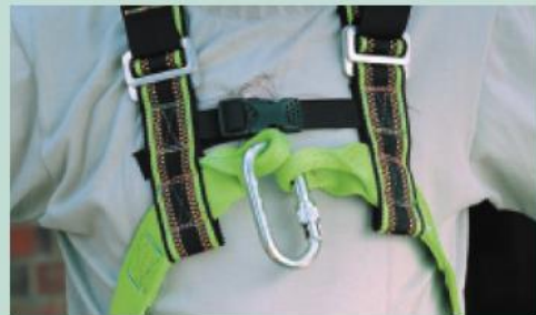
Front Anchorage Loops: The loops are connected using a karabiner. A fall arrest intermediate attachment is then connected to this. Used in a variety of climbing (with rope grabs), confined space, rescue and work positioning situations.
