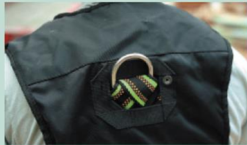
Rear 'D' Ring: The 'D' ring is the basic attachment point on a harness for fall arrest. It is suited to standard site work where the worker only needs to be attached for safety and does not need to work in suspension at height.
