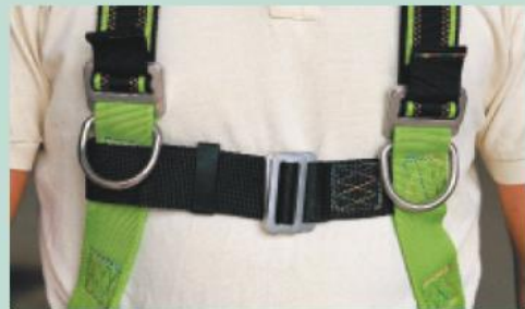
Front 'D' Rings: These are used together for fall arrest; a front attachment provides better control. Generally more comfortable to hang in, they may also be used in a rescue situation.
