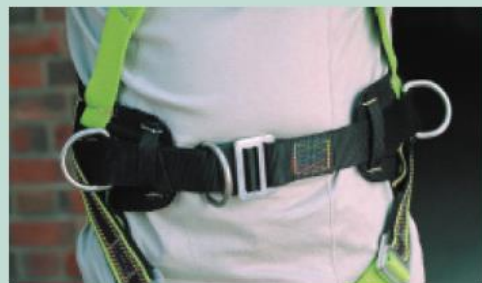
Side 'D' Rings on the Belt: These 'D' rings must not be used for fall arrest applications. Most commonly they are used for work positioning where the worker is required to be suspended for extended periods of time. The use of a belt enhances the comfort for the worker.
