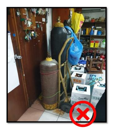
Gas cylinders stored indoors without proper ventilation
