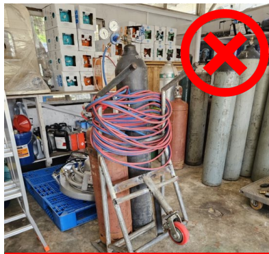
Unsafe storage of cylinders
