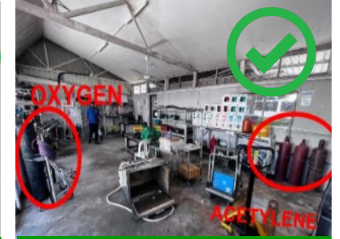
Segregation of combustible and explosive cylinders
